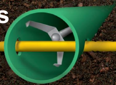
Natural gas pipelines installed using trenchless practices may have inadvertently penetrated sewer service lines.
