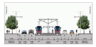
Figure A – Typical cross-section of an LRT stop<sup>1</sup>
