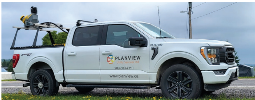
Planview's mobile LiDAR rig in action — capturing ultra-accurate 3D point clouds and 360° street imagery for seamless GIS.
